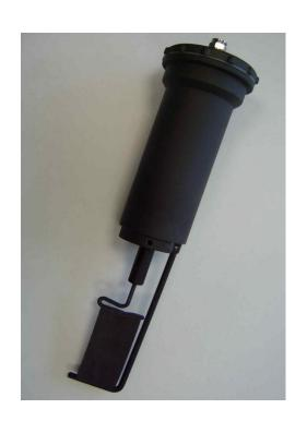
**OILSPY** is a hydrocarbons detector designed to generate an alarm in presence of accidental pollution.
